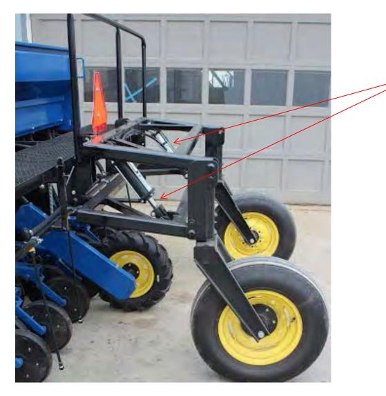
Insert cylinder stops here to assist with leveling if needed
